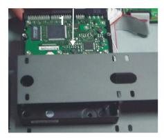
First, put the HDD into the HDD fixation rack sides
